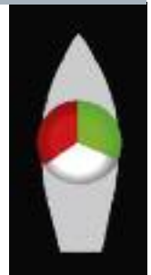
Sailing yacht under 20m tricolour lantern at masthead
