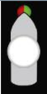
Motor boat under 12m, combined masthead & stern light
