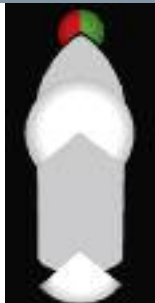
Motor boat under 20m, combined lantern for sidelights
