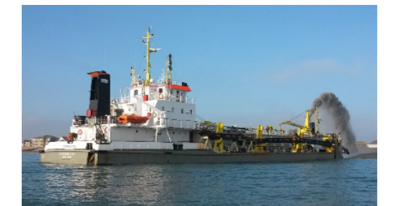
Disposing of the dredged sediment
