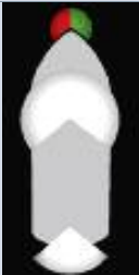
Motor boat under 20m, combined lantern for sidelights
