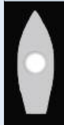
Sailing boat under 7m shows white light to prevent collision
