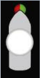
Motor boat under 12m, combined masthead & stern light
