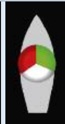
Sailing yacht under 20m or 20m tricolour lantern at masthead
