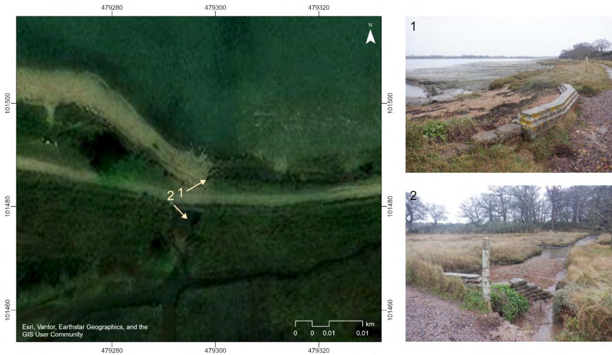
Figure 3.13. Hard structure along the footpath enabling the marsh landward of the footpath to be inundated at high tide.
